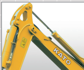
Bucket cylinder hose is placed inside of arm. Improves forward visibility and helps prevent damage to the hose.
